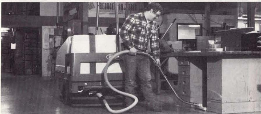
Water and spills can be vacuumed from hard-to-reach areas with Tennant Company's 530E scrubber attachment — the vacuum squeegee wand. The optional attachment plugs directly into the battery-powered rider scrubber, eliminating the need for separate equipment to clean under and around objects. The 530E is a fast, quiet, pollution-free model that includes a side brush and battery charger as standard equipment.
