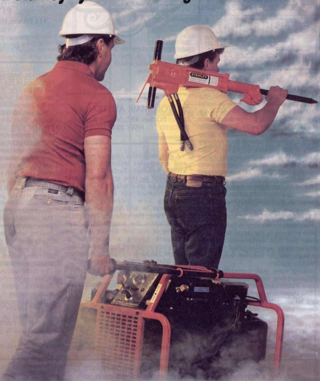
Hydraulic fluid transmits power more efficiently than air. So hydraulic-powered tools are lighter, and work harder than air-powered.
